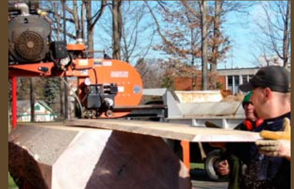
The Center's Wood-Mizer portable band saw mill
